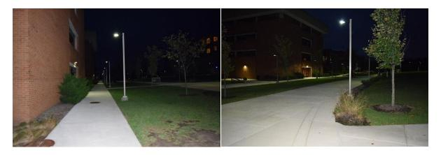
**ECS**: Pole lights are illuminated. The Pedestal lights are unserviceable. FM will take light measurements in this area and if pole lights are providing adequate illumination, we will remove the pedestal lights. Light readings to be taken next week.
